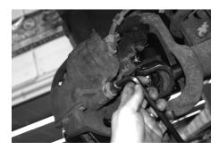
• NOTE FOR 00-01 models only!! Install the spacers provided between the caliper bracket and steering knuckle.
