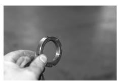
• Tighten the inner locknut to 50 ft/lbs, using a spanner locknut wrench and rotating the disc brake rotor & hub
