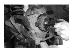
• Install the new outer stub axles to the inner axle shafts
