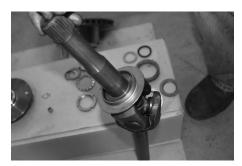
• Install dust shields, spacers & seals to the outer stub axle
