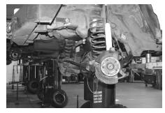
• Remove factory bolts retaining the unit bearing
