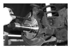
Make sure you install the dust shields prior to installing the spindle
