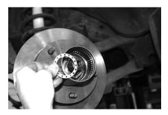
• Install the outer locknut, tighten to 160-205 ft/lbs
