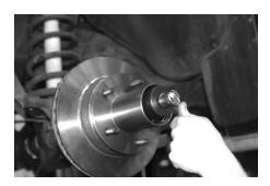
• Install lock washer. The key should be positioned into the groove of the wheel spindle. Tighten inner locknut, align the pin to the nearest lock washer hole
