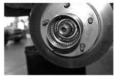
• Install the inner jam nut, with the pin facing outward
