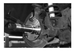
• Install the hub & rotor assembly onto the spindle. Be careful not to jam the bearings or damage any seal surfaces
