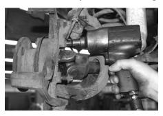
• Remove unit bearing assembly. This may take some force depending on amount of rust, salt or corrosion present
